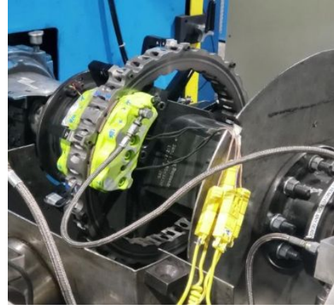
Brake test setup at Greening
