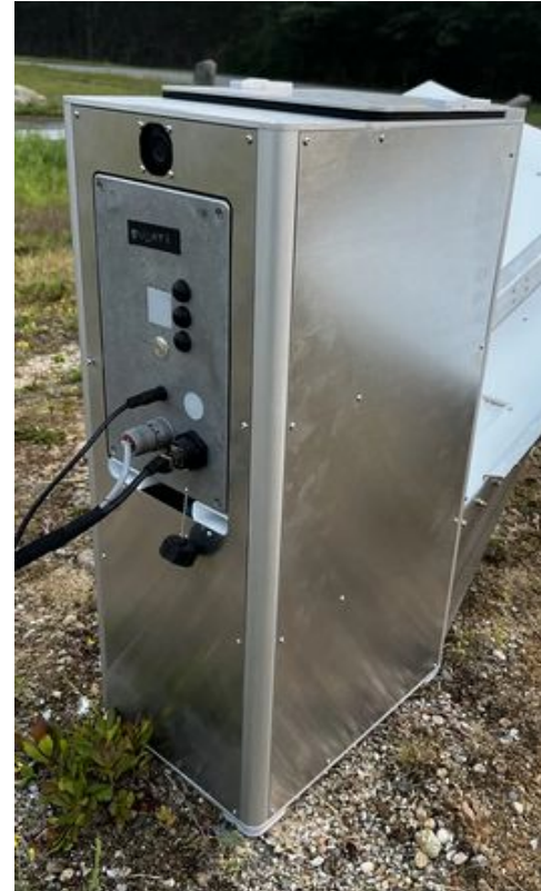
Dry box accessible from outside of hive
