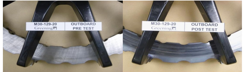
Picture of rotor pre and post test. Bell (black) holds onto outer edge of rotor
