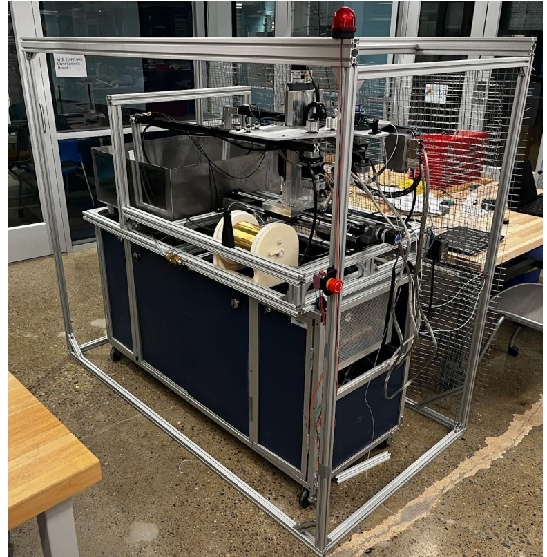
Complete WEDM machine with safety enclosure
